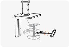
Remove the handscrew from the base assembly using the large Allen wrench.
