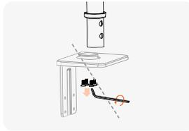
Use the small Allen wrench to remove the tube completely. You can set all other base assembly components aside.
