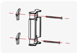
Attach the plaster wall mount screws and toggle bolts to the mount adapter.
