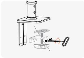
Remove the handscrew from the base assembly using the large Allen wrench.
